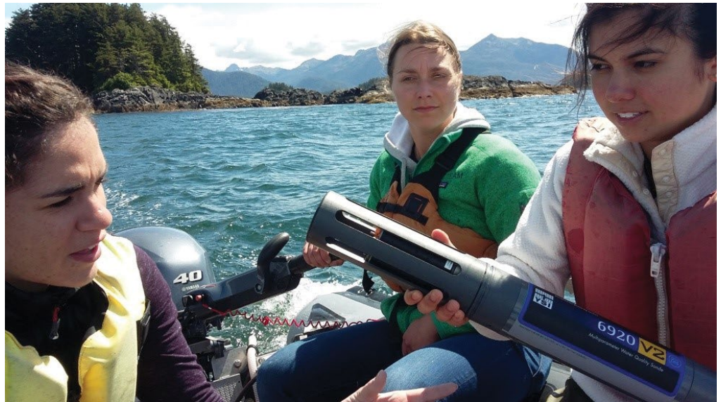
1/c Sydney Mills (left), Biologist Lauren Bell (center), and 1/c Eva Sandri (right) prepare a sonde to measure sea conditions within kelp forests in Sitka Sound, Alaska.
