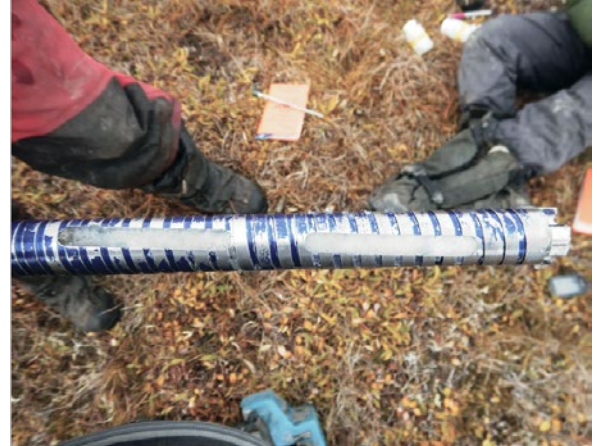
Left, Cordell Johnson drilling and coring the interior of the bluff to ground-truth geophysical methods. Right, a core section filled mostly with ice.
