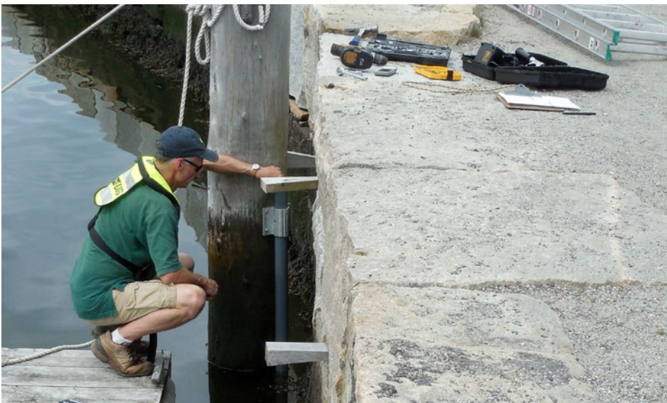
Craig Brown , a USGS hydrologist, installs a sensor pipe for the SWaTH Network.
