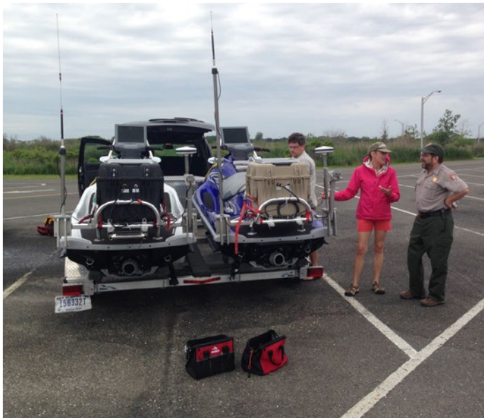
USGS research geologist Cheryl Hapke (center) explains to National Park Service manager Mike Bilecki (right) how instruments mounted on personal watercraft will measure depths in shallow water. USGS engineering technician BJ Reynolds is beside the watercraft.
