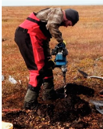
Left, Cordell Johnson drilling and coring the interior of the bluff to ground-truth geophysical methods. Right, a core section filled mostly with ice.
