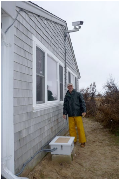
Chris Sherwood poses below the Sandwich beach camera. The white box contains a small uninterrupted power supply.
