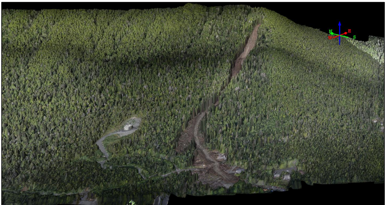
Figure 1. Orthophoto mosaic draped over the DSM created from SfM photogrammetric methods shows an oblique view of the South Kramer debris flow on August 20, 2015.
