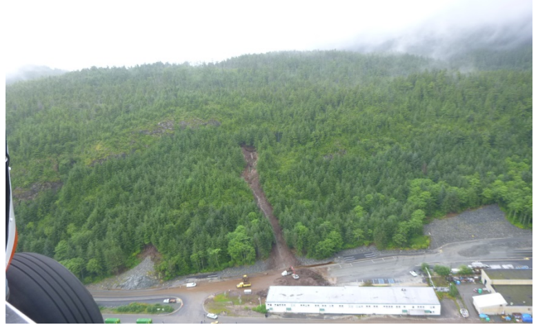
Photo 6 – Aerial view of debris flow at the Gary Paxton Industrial Park, (Source: US Coast Guard)
